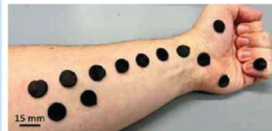
Play putty for flexible biometric sensors (Credit: https://www.umass.edu )
